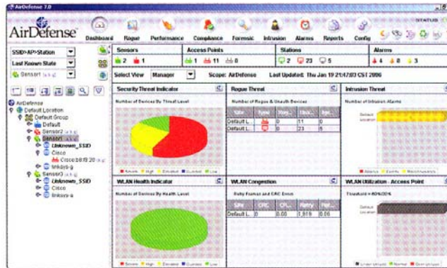
AirDefense Enterprise has redesigned its dashboard by grouping its core functionality into five analysis wizards—rogue, performance, compliance, forensic and intrusion.
